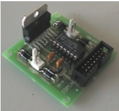
The H-bridge board allows the actuation of two DC motors.
