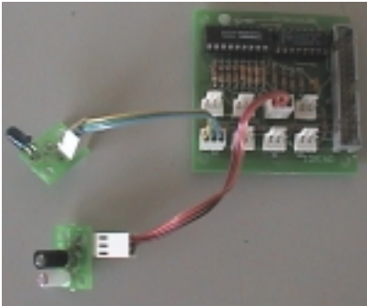
Analog interface board for 8 analog sensors (emitter/receiver). In the figure this board is connected to two sensors: One board with an IR receiver and another board with a green led and an LDR.
